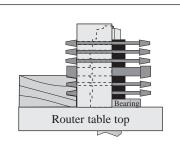
Finger Joint Bit Shown Cutting A Max. 5/8" Wood Stock
