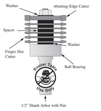
The cutters cutters should always be assembled to match spindle rotation. Be sure to use a spacer between cutters at all times!
