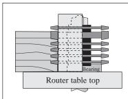
Finger Joint Bit Shown Cutting A Max. 1-3/16" Wood Stock
