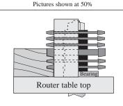
Finger Joint Bit Shown Cutting A Max. 13/16" Wood Stock
