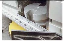
(TOP) Align the centreline of the stock with the centre of the upper bevel as shown.
