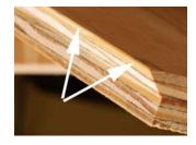
2. Install the larger diameter bit and set its height to <sup>3</sup>/<sub>4</sub>". Set the fence so that roughly <sup>1</sup>/<sub>4</sub>" of the bits cutting edge is ahead of the fence faces. As with the smaller bit, make test cuts and adjust the fence back until the miter edge nears a knife edge but has a very narrow flat along that edge.
